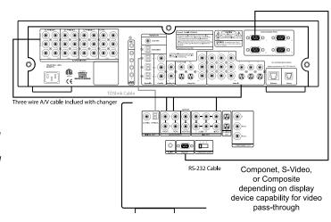
FireBall requires that you connect each changer to the back panel using audio and control cables.
